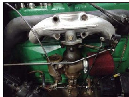
Carby reconfigured because turning the carby alone would have the throttle valve and choke controls the wrong way around.
