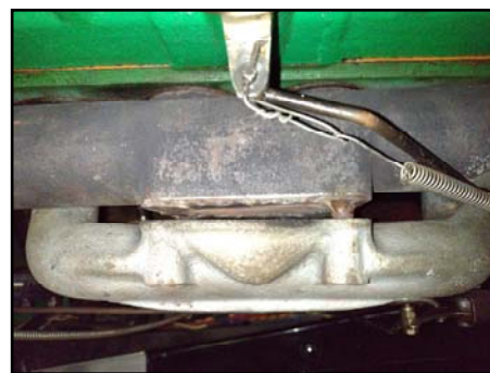
Inlet manifold now virtually "air gapped" from exhaust manifold. Original exhaust flame front is directed onto the inlet manifold with no thermatic deflector.
