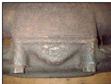
Original exhaust flame front is directed onto the inlet manifold with no thermatic deflector.
