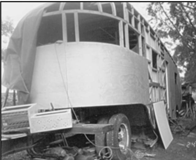
*Although this was taken a bit earlier, it shows the complexity of the front of the caravan. There is a simple curve for the main wall, but the curve of the roof meeting the square box section of the main van presents many headaches.*
